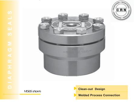
The Trerice Drop-In Welded Diaphragm Seal is furnished with a Clean-out design for use on piping 4" or larger in diameter. The diaphragm seal is installed by welding the process housing directly into the pipe. Available diaphragm choices include: Teflon (T), Viton (V), Removable Metal (M) and Welded Metal (W).
