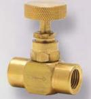
Brass, 1/4" NPT female connections only. Suitable for 600 psi at 300° F maximum; for water, oil or gas service.
