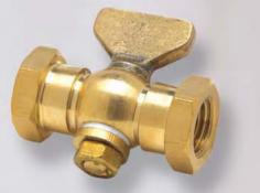
In polished brass for pressures to 200 psi hydraulic, 1/4" NPT female connections with hex shoulders.
