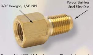
Brass with 1/8" thick micro-metallic stainless steel filter (max pressure 1500 psi) Available 1/4" NPT only. Models available for air only, or water or light oil only. Both are Stainless steel body instead of brass.
